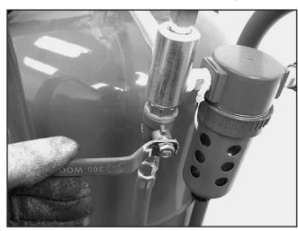
Figure 9. Blast hose air supply valve, closed.
